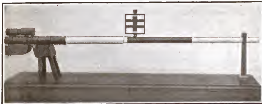
Fig. 4.—Sample of flashlight barrier for grade crossings
